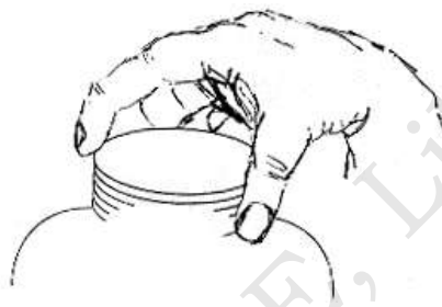
Fig. 2.15. Our fingers apply a couple to turn the lid
